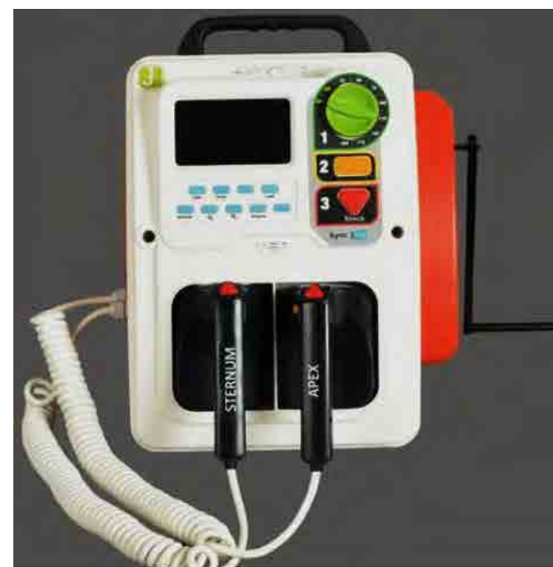
Hand Cranked Defibrillator for Sudden Cardiac Arrest
