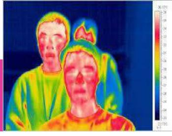
Facial Temperature of all people walking into a facility is measured remotely using a thermal camera.
