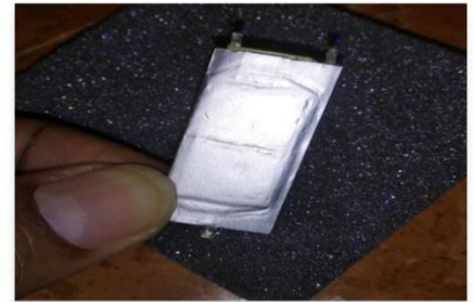
Pouch Type 5mF Carbon Supercapacitor - Prototype
