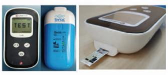
PathShodh Healthcare Pvt. Ltd. has developed anuPath LiTe, which is a Self-Monitoring Glycaemic Control Device (SMGC) based on cutting edge patented technology. The device is capable of measuring three important biomarkers (Blood Glucose, HbA1c and Glycated Albumin) in finger prick blood sample which gives a comprehensive diabetes management. The device has been extensively validated and the Company has all regulatory approvals in place for the product.
