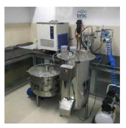
15 Kg Bioreactor with automation developed by Fermentech Labs Pvt Ltd for the production of phytase enzyme
