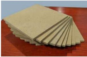
Finished Fibreboards developed by Western India Plywood Ltd using Paper Mill sludge
