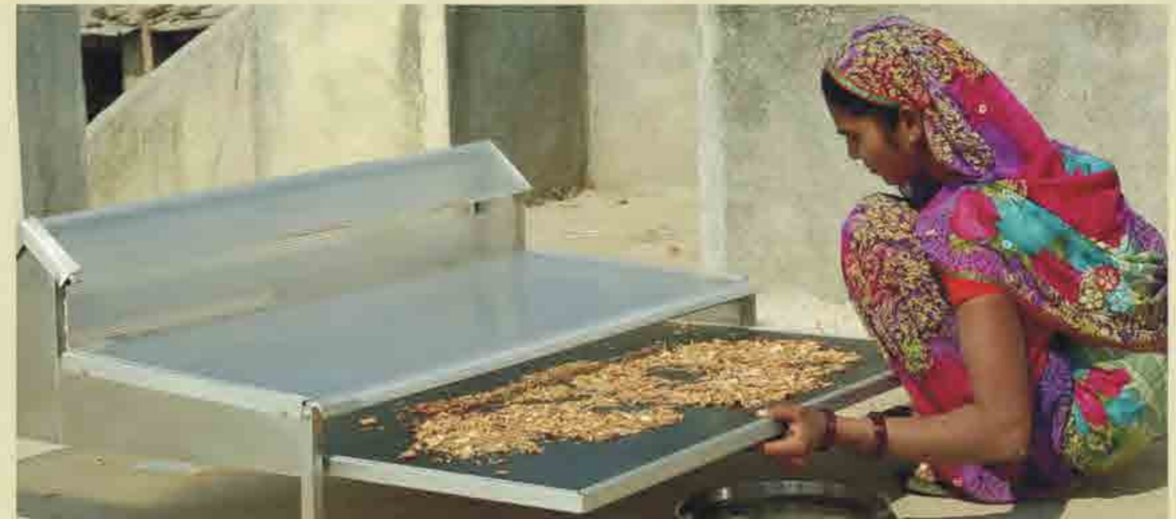
»»» The Solar Conduction Dryer being used by a beneficiary from the pilot study of Science for Society, Maharashtra, under the Achieving Health Growth through Agriculture and Nutrition call under Grand Challenges India
